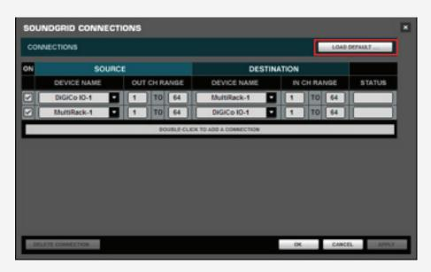
You can create connections manually or use the **Load Default** button to load "32 Racks Processing." Remember to turn Individual Connections ON.
