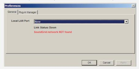
When set correctly, **Link Status** is UP, **Link Speed** is 100 Mbps, and you will see the "SoundGrid Network Found" message.
