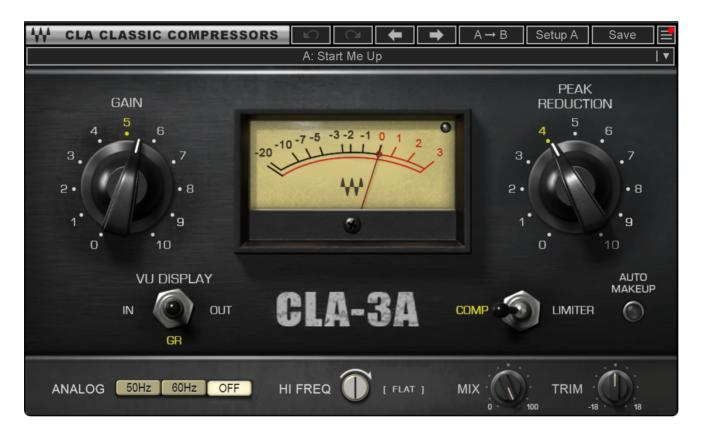
The CLA-3A offers two main controls for compression, as well as additional controls for fine-tuning.
