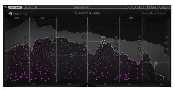
The graphic analyzer display shows the input and output levels of the neural network, as well as the difference between them (reduction). The display is divided into six frequency bands whose ranges are set with draggable crossovers. Each band has a Band Process fader that is used to offset the processing of Main Control knob processing. As you drag a band's process control downward, you reduce the neural network's process strength for that band and bring back some of the ambience.
