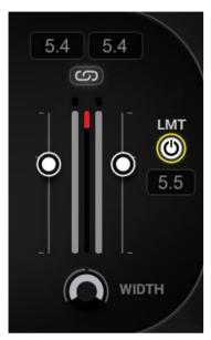
Full-scale meters (stereo or mono) indicate the plugin output. Peak hold values are shown above the meters. A red clip LED indicates a level of 0 dBFS. Click on the meter to clear peak hold and clip indictors.
