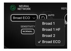
There are four Clarity Vx Pro neural networks. They differ in the statistics, signal-to-noise ratios (which were introduced to it during training), and weights and biases (which they apply during processing). Choose a network based on the input source, as well as the voice focus that you are seeking.
