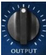
**OUTPUT** controls the output level.
