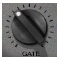
**GATE** controls the gate threshold.
