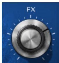
**FX** controls the track's FX send gain.
