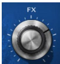
**FX** controls the track's FX send gain.
