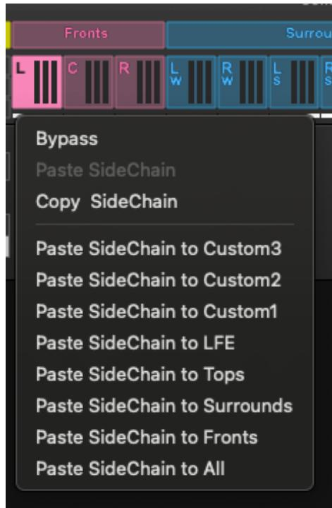
**Sidechain Receive Settings** – When the Internal sidechain mixer is open, the **right click** functionality on the channel buttons will change to allow you to copy the sidechain receive faders setting to other channels or groups of channels. Use this to align channels to the same settings and eliminate relative control positions.
