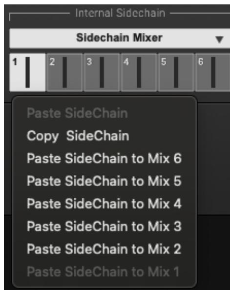
**Sidechain Sends Settings** – **Right click** on one of the Internal Sidechain Mixes to copy its channel sends to other mixes. Use this to align channels to the same settings and eliminate relative control positions.
