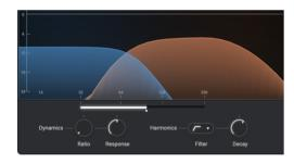
The third position provides a 24 dB per octave rolloff at the selected Frequency. This position is a good starting point for situations where you are mixing for a specific small speaker system. It removes almost all very low frequencies from the Harmonic output, allowing greater levels while reducing the risk of pushing the transducer too far.
