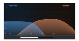
The MaxxBass Graph illustrates the Original Bass sound (blue) and the generated Maxx Bass sound (orange). The Frequency slider controls the crossover point. All frequencies below this point will have harmonics created for them; all frequencies above this point will be passed to the output unaltered. The Highpass Filter Selector sets the slope of the MaxxBass signal.
