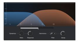
The middle position (default) provides a 12dB per octave rolloff at the selected Frequency, and is ideal for most mastering situations.
