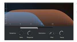
The wideband filter leaves a large portion of the generated bass signal unaltered, extending all the way to DC. It can be used for extreme effects where a hyperextension of the low frequencies is desired.
