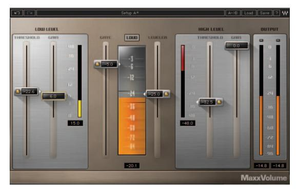
The MaxxVolume interface is organized around the central Energy Meter. The controls are laid out so that Low Level signal functions are on the left side of the interface, while High Level signal functions are on the right side of the interface.
